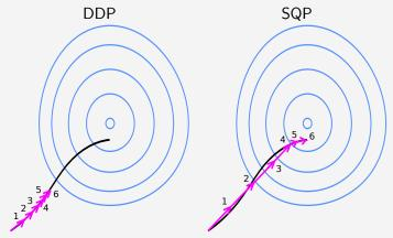
Nonlinear rollout (DDP) does small steps due to constraint satisfaction
